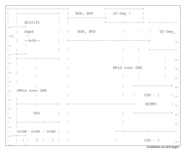
Using publicly available BFD implementation, BFD Daemon (BFDD) would be integrated with QBGP. In this approach, the BFDD would make use of BFD messages to detect the health of the connection with the DC-Gwy.
