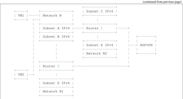
Network N gathers 2 subnetworks, subnet A IPv4 and subnet B IPv6. This makes possible to create Neutron Ports, which will have 2 IP addresses and whose attributes will inherit information (extraroutes, etc) from these 2 subnets A and B.
