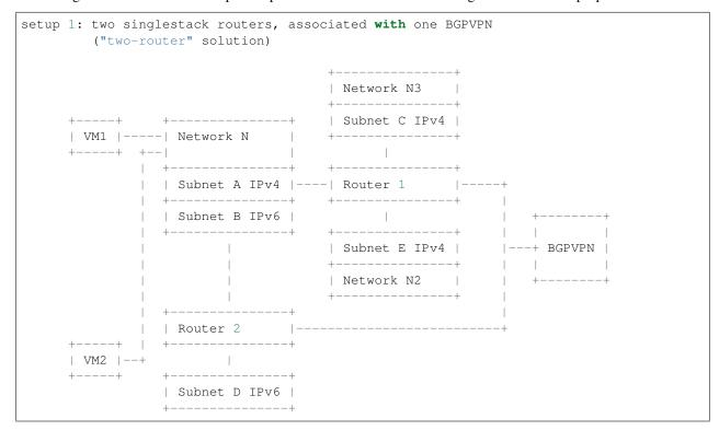
Network N gathers 2 subnetworks, subnet A IPv4 and subnet B IPv6. This makes possible to create Neutron Ports, which will have 2 IP addresses and whose attributes will inherit information (extraroutes, etc) from these 2 subnets A and B.
